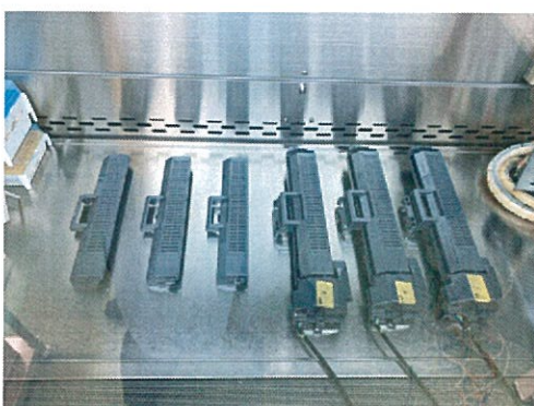
Picture.3 Installation of test carrier
