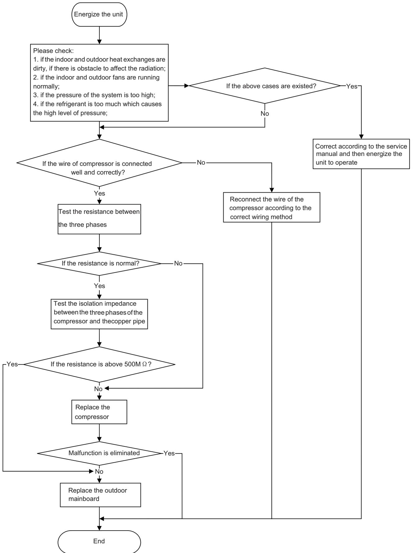
2. PFC protection malfunction, capacity charging malfunction
