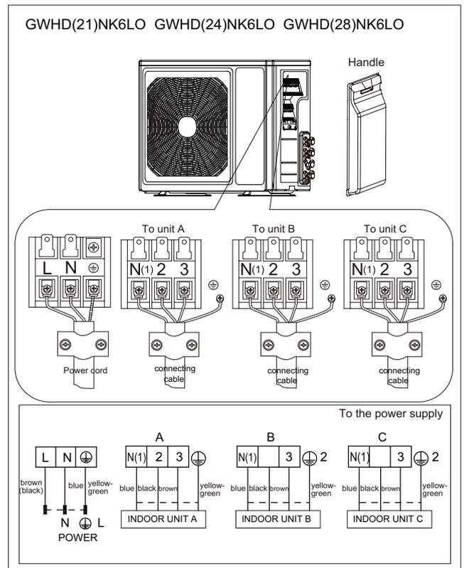
**!** An all-pole disconnection switch having a contact separation of at least 3mm in all pole should be connected in fixed wiring.
