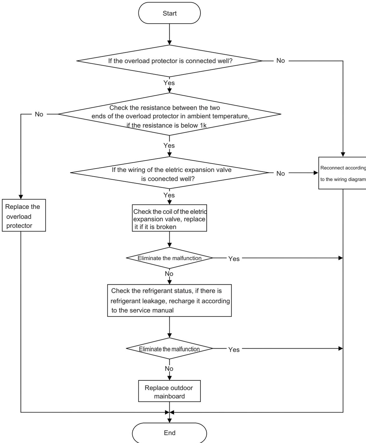
Note: the detection method of the coil of the electric expansion valve: there is five pieces of coil of the electric expansion valve, the resistance of one of them (the leftmost or the rightmost one) is almost the same as the resistance of other terminal (within 100 Ω ). Judge the condition of the electronic expansion valve through detecting these resistance.
