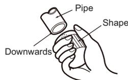
**C: Put on suitable insulating pipe**
