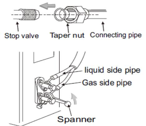
★When prolonging the piping, extra amount of refrigerant must be added so that the operation and performance of the air conditioner will not be compromised.
