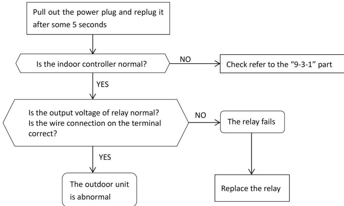
④The Step Motor Does Not Work
