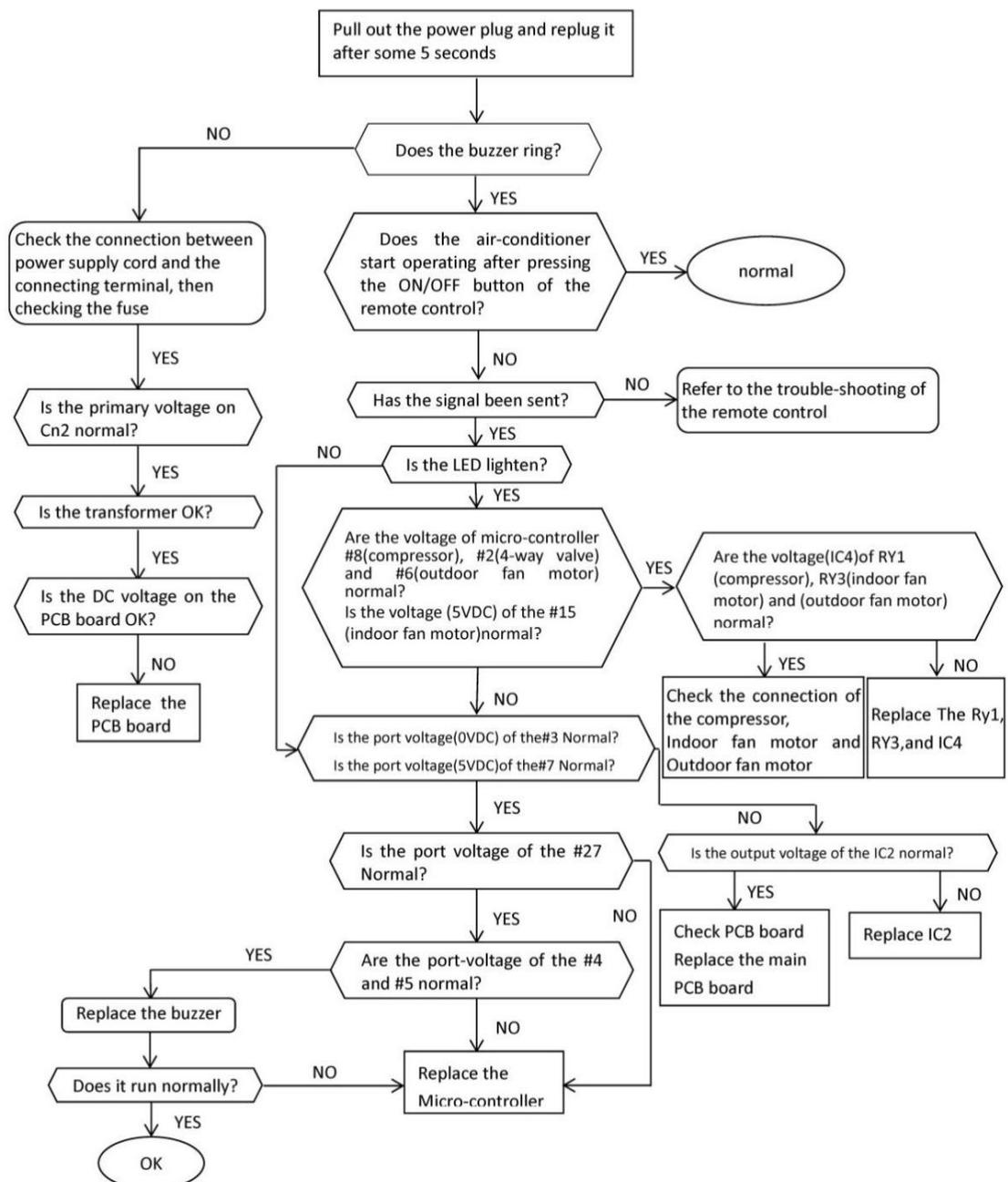
②The Indoor Motor Does Not Work
