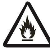
Please notice that the unit is filled with flammable gas R32. Inappropriate treatment of the unit involves the risk of severe damages of people and material. Details to this refrigerant are found in chapter "refrigerant".
